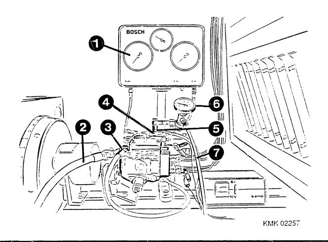
ATTACHMENT OF TIMING-DEVICE MEASURING INSTRUMENT
